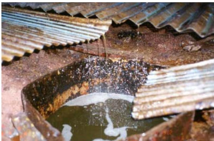
Final stage of collecting resin filtered through bags, quality is suitable for export
